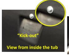
8.2: Secure the tub to the aluminum frame using the 1 3/4" bolts, nuts and washers. Make that the washers are installed inside the tub in direct contact with the plastic as pictured.
