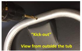
8.1: Make sure that your tub is centered within your frame and drill a hole above the two tub kick-outs (back and front of the cart) going through the pre-drilled holes in the aluminum frame. You would need a ¼" size drill bit and a powered drill.
