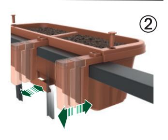
Attach railing bracket from below planter sides and middle at the desired width.
