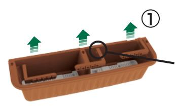
Remove railing brackets, pins & metal clip from drainage tray: 3x railing brackets, 3x pins, 1x clip **IMPORTANT**: You will find locking pins nested in railing brackets.
